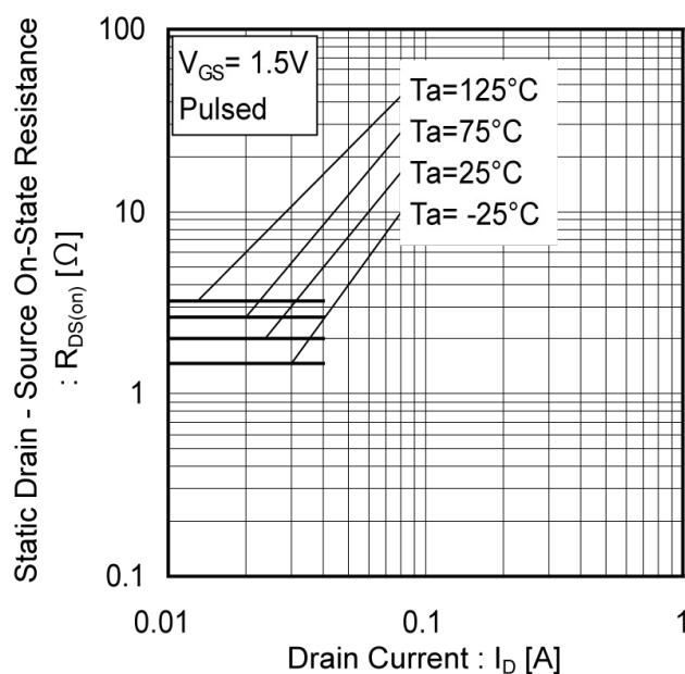
Fig.16 Static Drain - Source On - State
