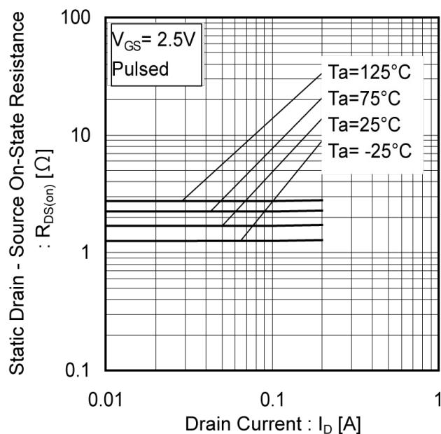
Fig.14 Static Drain - Source On - State
