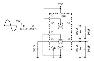
Figure 6 Cross Talk (between any two switches)
