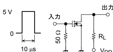
$V_{DD} = 5\text{ V}$
